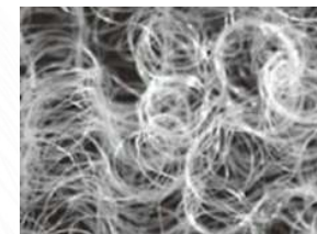
Natural crimped structure of the fiber
